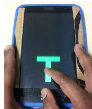
Figure 2. Subject tracing stimuli displayed on the touch-based device with the vibro-audio mode.
