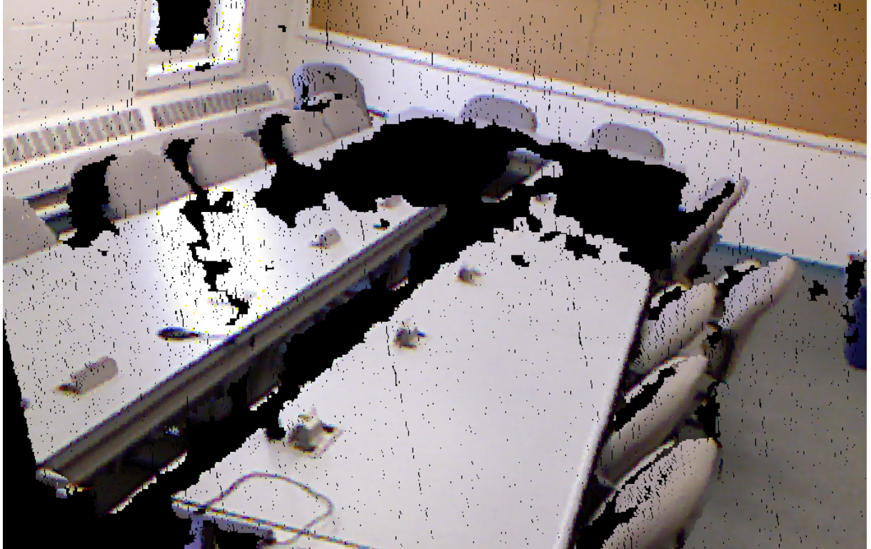
Figure 2.3. Gaps in a point cloud due to the properties of a table's surface
