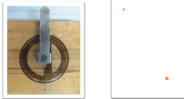
Figure 4.6. Pointing device used in the pointing task (left) and A4 Canvas for reconstruction with start and destination points(right)
